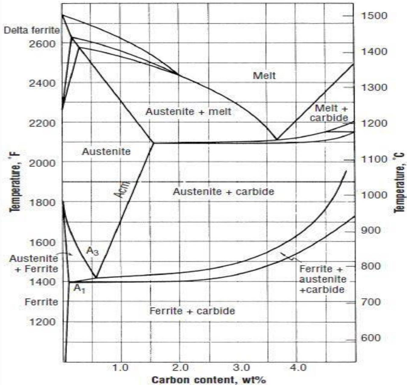
**Fig 2. Fe-C-Si diagram at 2% silicon.**
