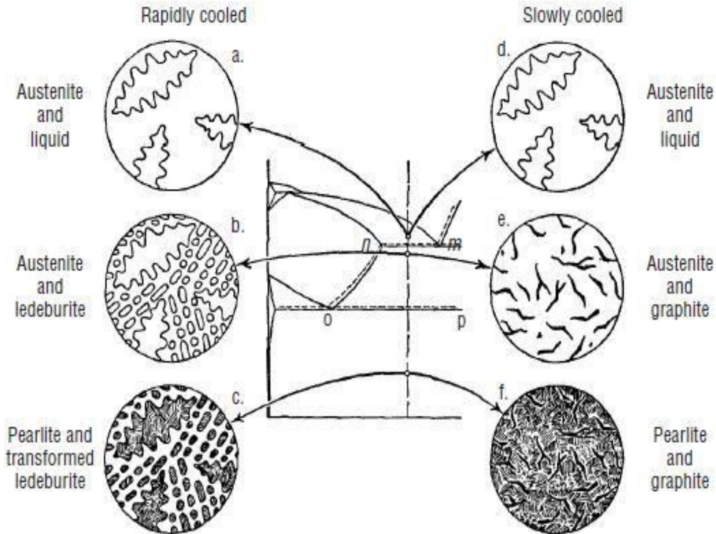
**Fig 3. Iron-graphite phase diagram [4]. Microstructures obtained by cooling and solidification of cast iron; white iron (left) and gray iron (right).**
