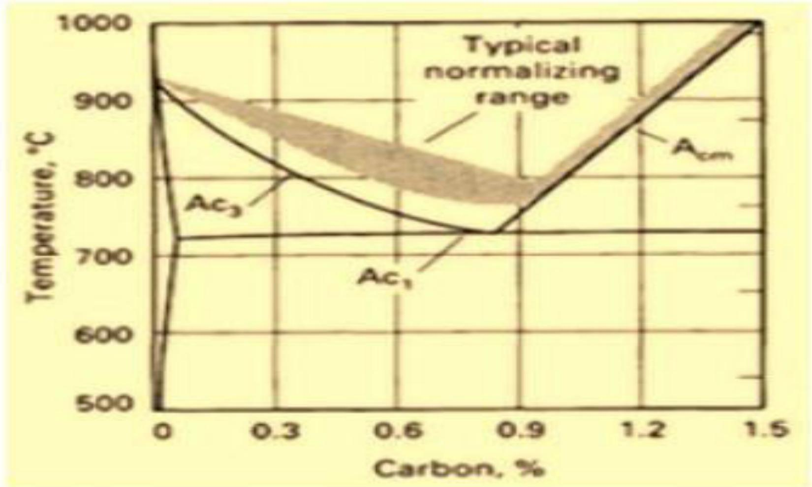
Fig 1 Typical normalizing temperature range for steels
